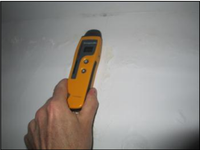
Test of water damaged area shows normal moist
